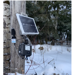
Noise and Vibration Meter powered with a solar panel. The unit measures noise, overpressure and vibration at regular intervals to monitor the general effects of mine site activities and prevent impacts to sensitive locations such as nearby residences, McLeod Park as well as waterbodies frequented by fish and other aquatic life.
