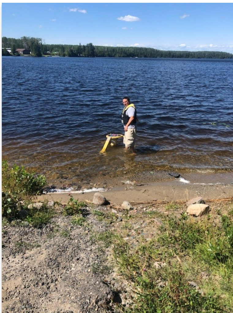
Randy Vernier measuring water flow using an Acoustic Doppler Current Profiler
