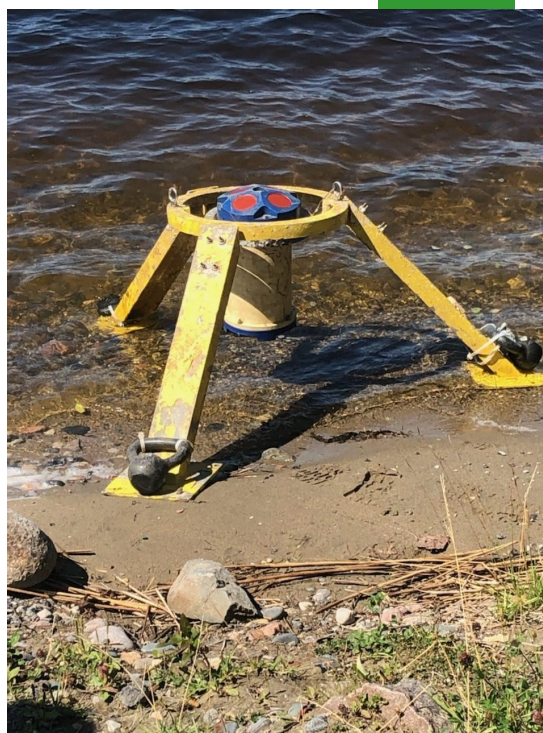
Randy Vernier measuring water flow using an Acoustic Doppler Current Profiler
